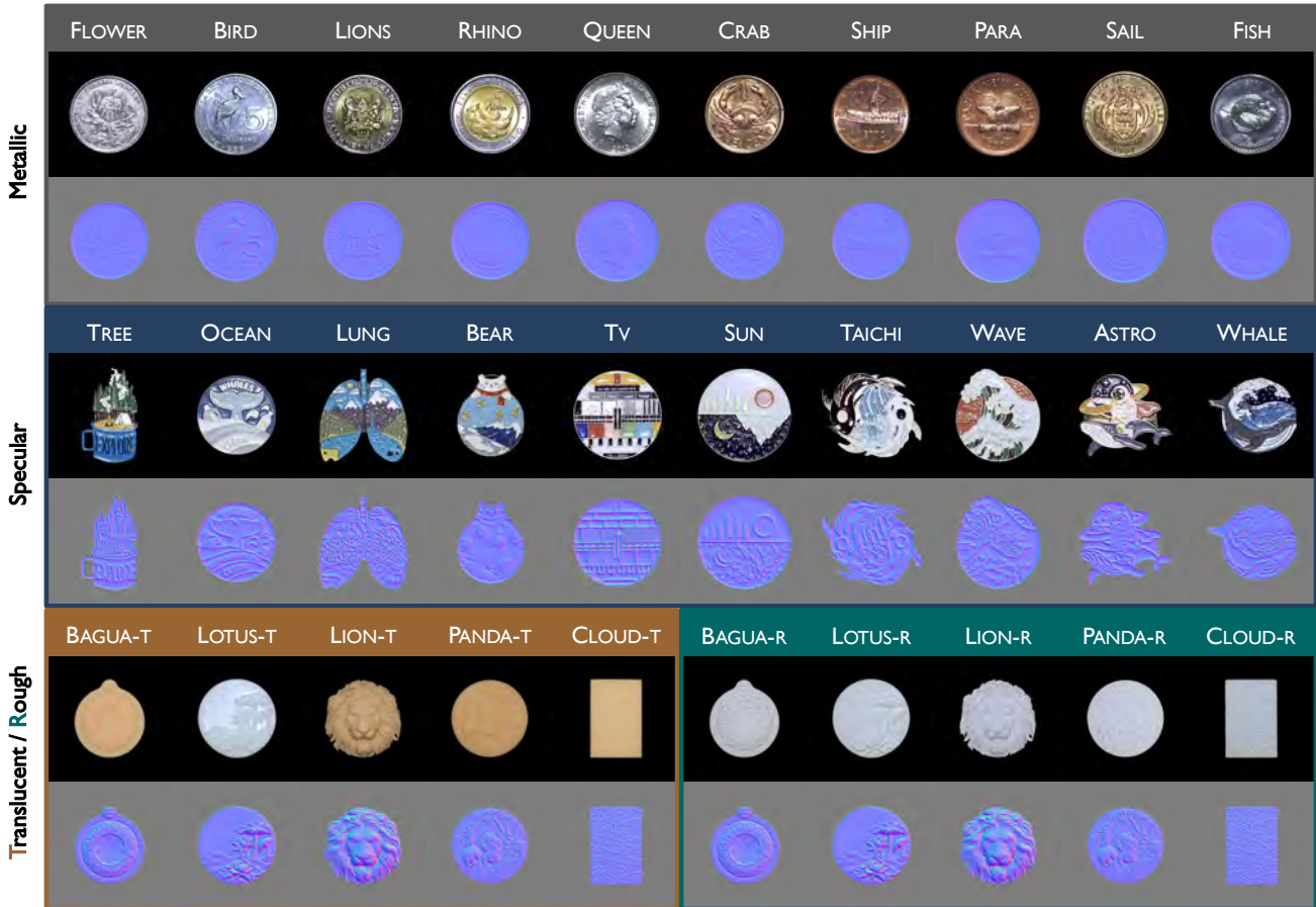
Figure 1: Overview of DiLiGenT-II. We collect 4 groups of near-planar objects with rich surface details and diverse reflectance types (metallic, specular, rough, and translucent). The corresponding ‘ground-truth’ surface normals shown in the even rows are measured via a precise profilometer in the accuracy of nanometers.
