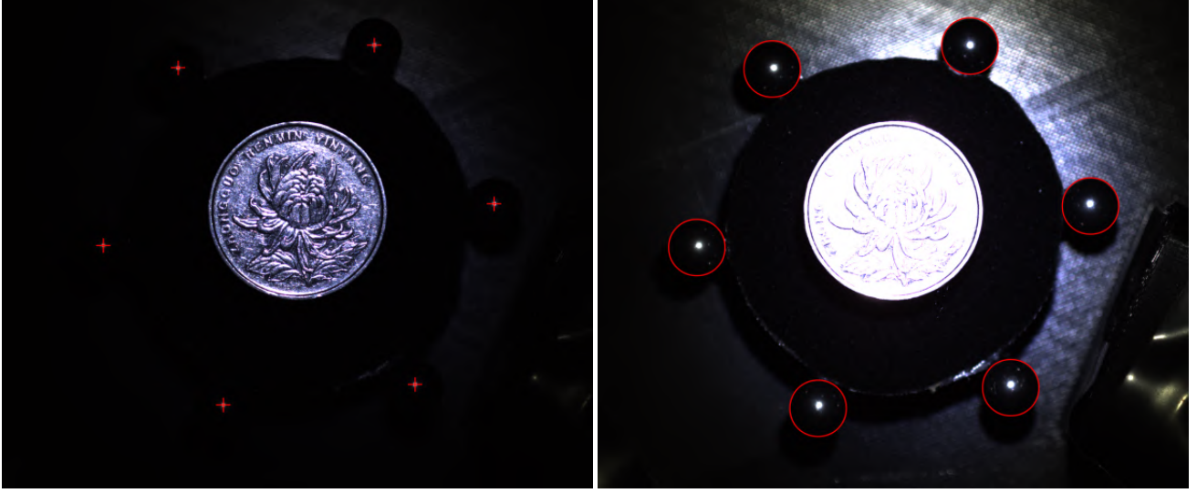
Figure S3: Images of FLOWER captured in low (left) and high (right) exposure time for detecting the specular spots and contour of the 6 mirror spheres for light calibration.
